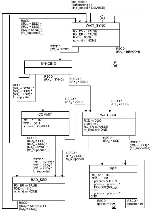
Figure 168–9—PCS Receive state diagram, part a
