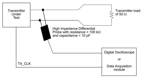
Figure 168–15—Transmitter test fixture 1 for transmitter voltage, transmitter droop, and transmitter timing jitter
