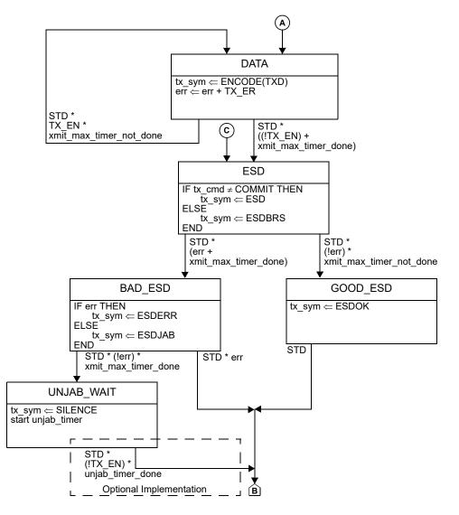
Figure 168–7—PCS Transmit state diagram, part b
